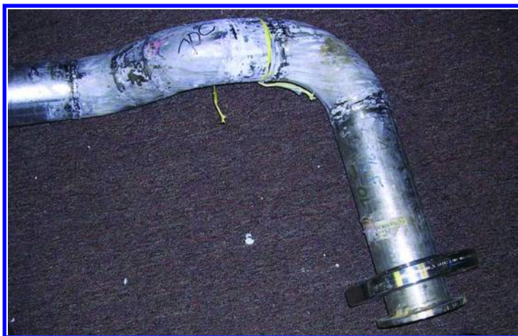
Figure 4. Pipe in >95% HNO 3 70 °C Service. Corrosion is seen in between and along welds (white area). (see color insert)
