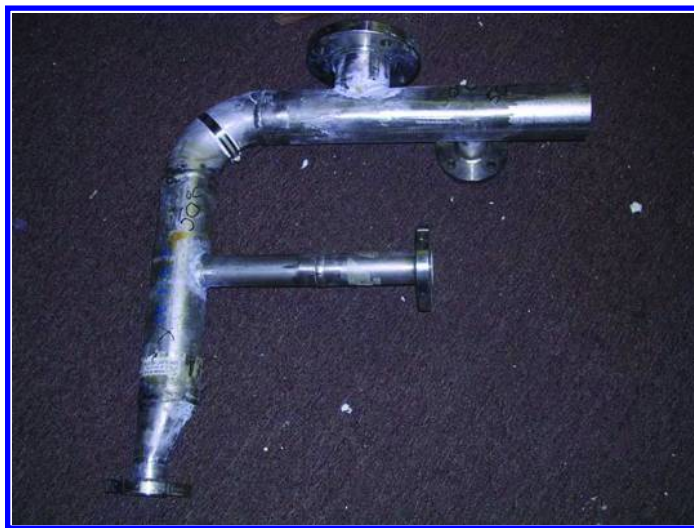
Figure 5. Pipe in >95% HNO 3 50 °C Service. Note the corroded areas are less extensive. (see color insert)
