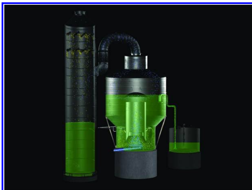
Figure 2. Interior view of the scrubber, neutralizer and rundown tank. Green indicates the ammonium nitrate solution, blue the ammonia and yellow the nitric acid. The spargers are on the outside of the draft tube. (Courtesy of Roland Huet). (see color insert)
